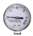
Do you own a dial gauge pressure canner? If you have a pressure canner with a dial gauge similar to the one pictured, it is important you have it tested for accuracy each year. We have a testing device at our office, and we offer this service to our
